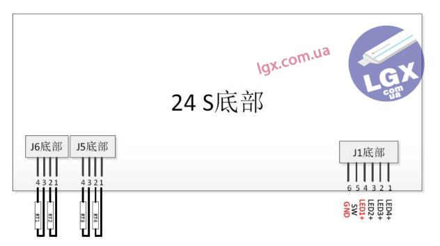
J5 and J6 for temperature sensor J1 for switch ( on/ off switch), use GND and SW signal.
