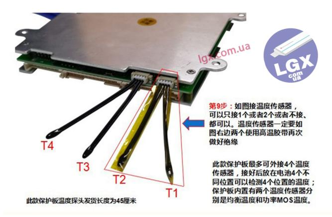
It is recommended to wrap the NTC with high temperature insulating glue for good insulation
